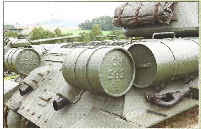
Rear section of the hull of a Czechoslovak T-34-85 with external fuel tanks. Note wide hinges on the rear armoured plate (6-segment, not 5-segment as the Soviet ones).
