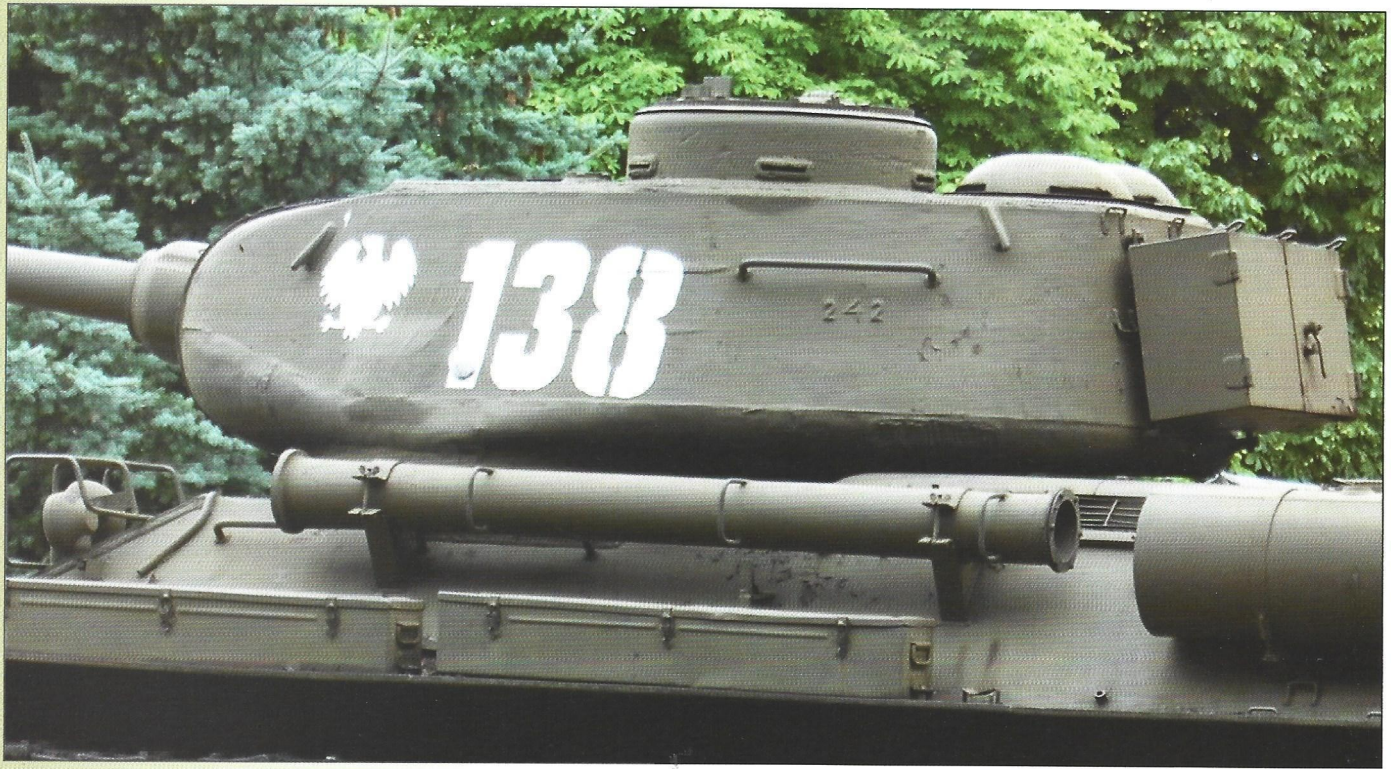
Above: Turret and middle section of the hull. The stowage box on the back of the turret and the snorkel are visible.
