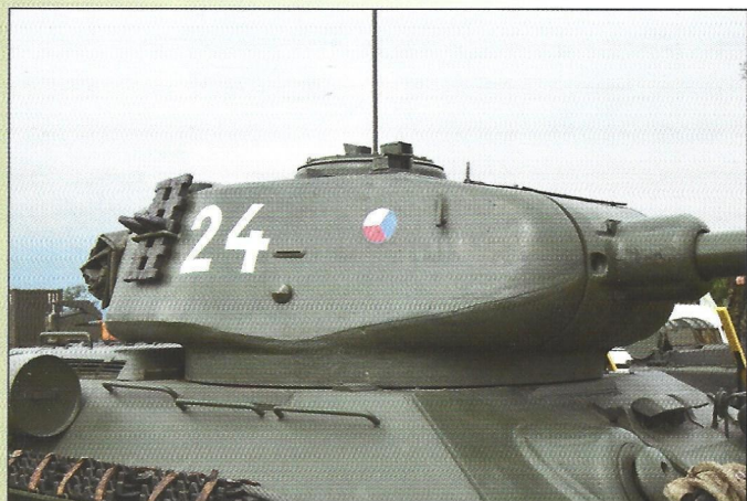
Details of the turret of Czechoslovak production. Note the quality of the casts and additional antenna mount on the turret roof.
