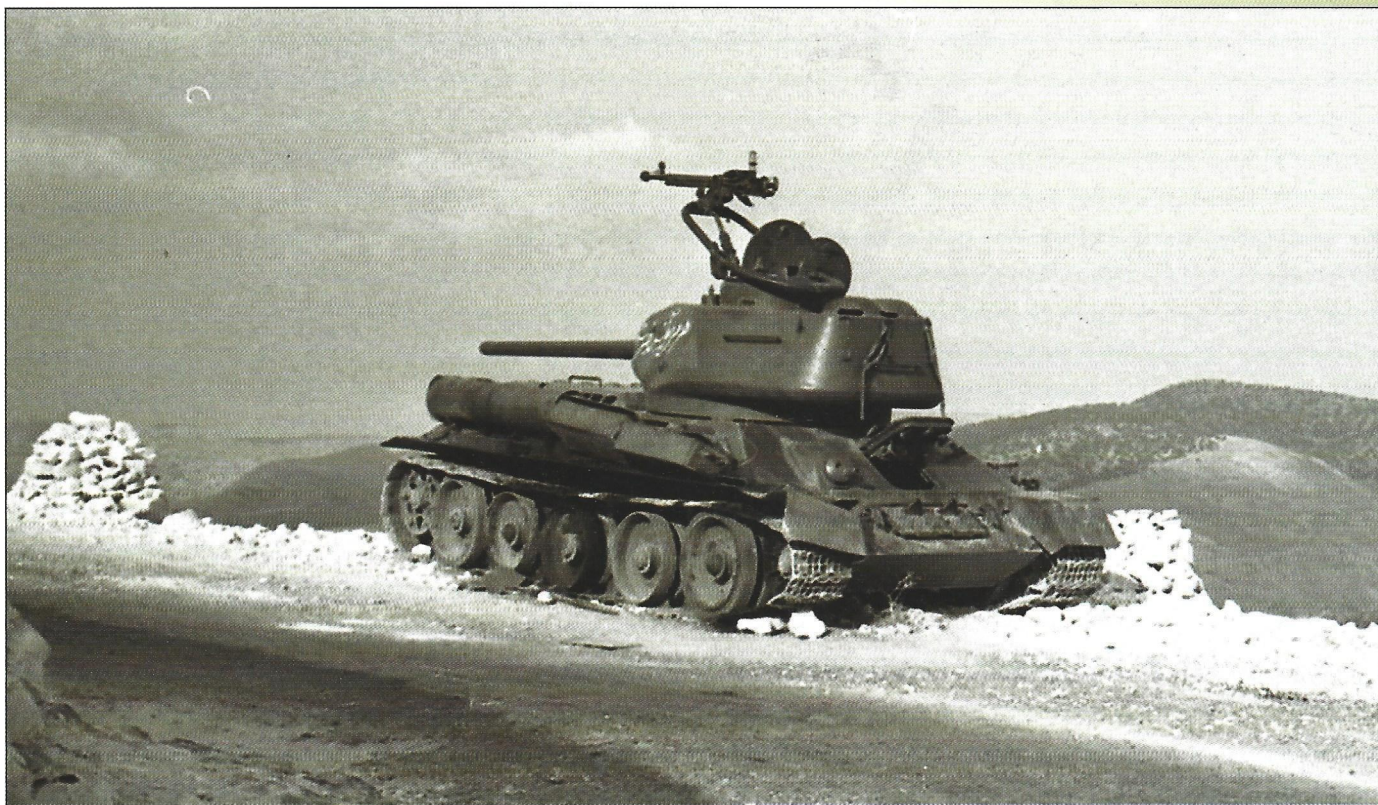
A Syrian T-34-85 (Czechoslovak production) lost during the Six Day War in 1967. The rail with grip for 12.7 mm DShK machine gun, characteristic for the Syrian tanks is well visible. The condition of the wheels indicates that the tank was burnt.
