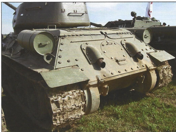
Rear section of the hull of another T-34-85 of Czechoslovak production with narrow hinges.
