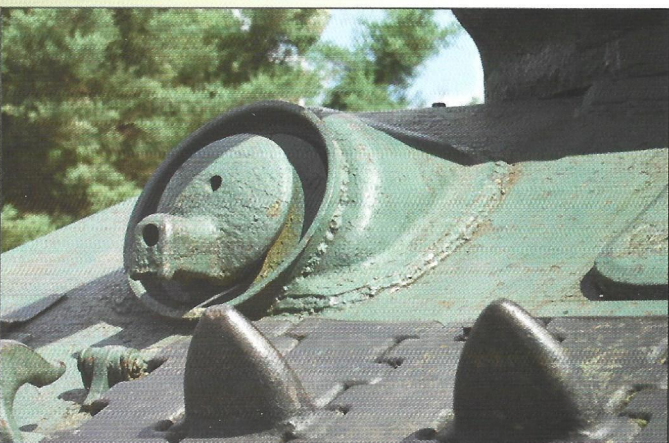
Forward machine gun with yoke enabling sealing.
