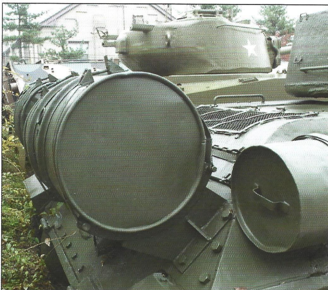
Below, below right: Holders for 200-litre barrels on the back of the hull.
