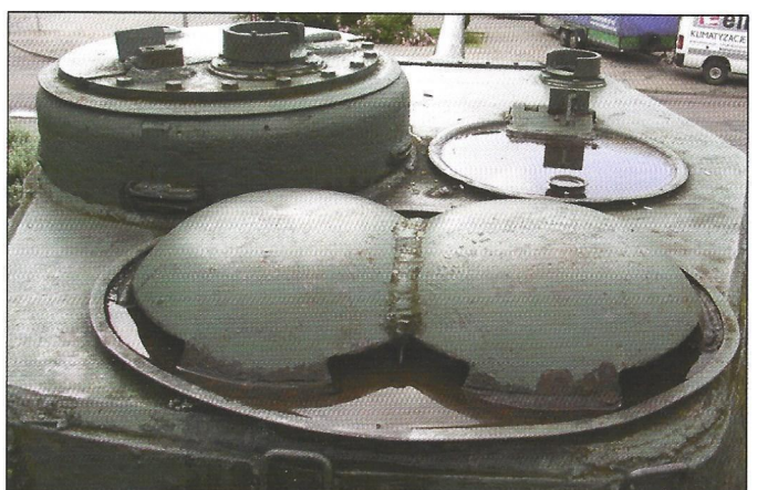
The roof of the turret with modifications enabling sealing and installation of the snorkel.
