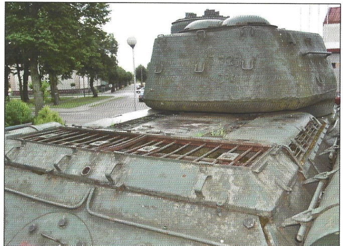
Rear section of the hull with louvres enabling sealing the engine compartment.
