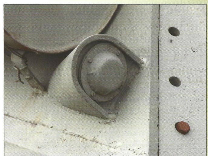
The signaling device for communication between the desant and crew characteristic for tanks of Czechoslovak production.
