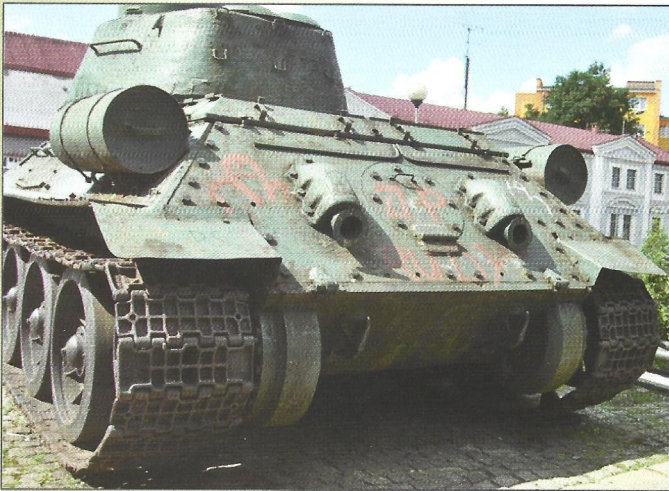
Rear section of the hull – fittings for cutoff valves on the exhaust pipes are visible.
