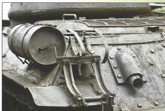
Rear section of the hull with holders for BDSH smoke canister and 200-litre fuel drum.
