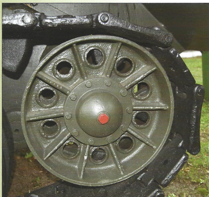
Below, right: Idler wheel of a Polish T-34-85.
