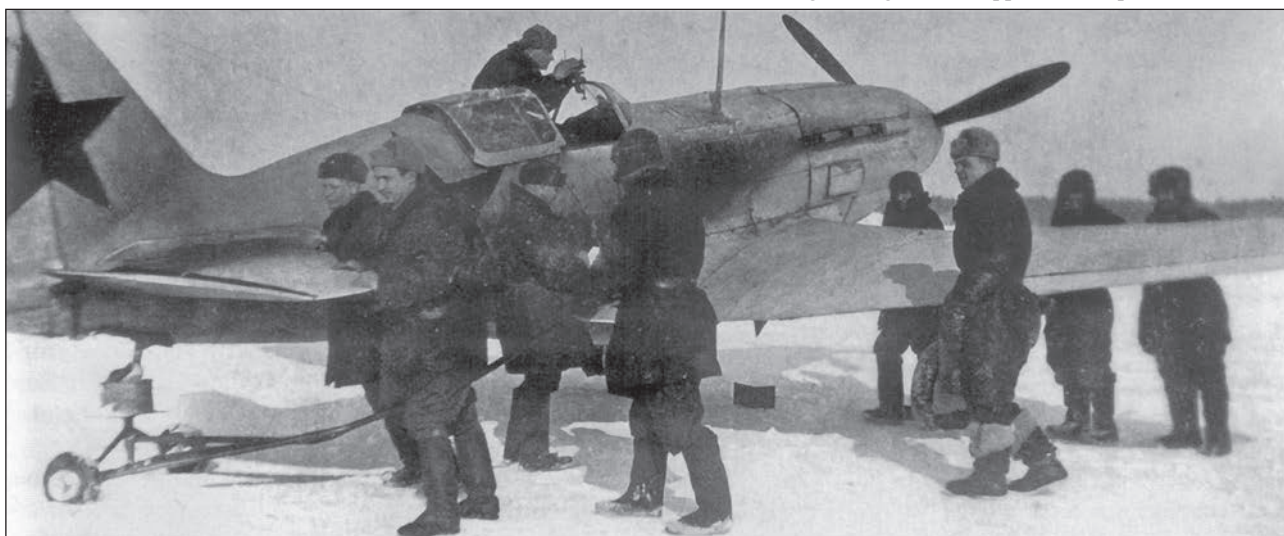
Left and below: MiG-3 of the 6th IAK of the Air Defense Forces, winter 1941–42. The airplane upper surfaces were painted in white throughout, the enlarged insignia were applied in six positions.
