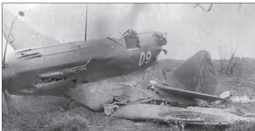
MiG-3 s/n 4809, tactical number 09, of the 169th IAP. On 3 October 1941, the airplane flown by Junior Lieutenant Kalinin was lost in a crash. The fighter was painted in monochrome 'protective' green colour on upper surfaces, with enlarged insignia applied in six positions. (20)
