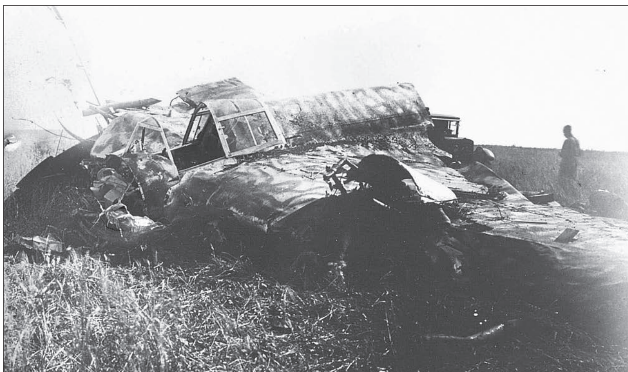
Wreckage of SB s/n 39/8 (built by Factory No.125), tactical number 7, from the 1st Squadron of the 32nd-A SBAP, which crashed at Balashov airfield on 8 August 1941. The airplane was painted in so-called 'Khalkhin-Gol' camouflage over its basic silver colour. Note the different paints used – most likely green and black. (8)
