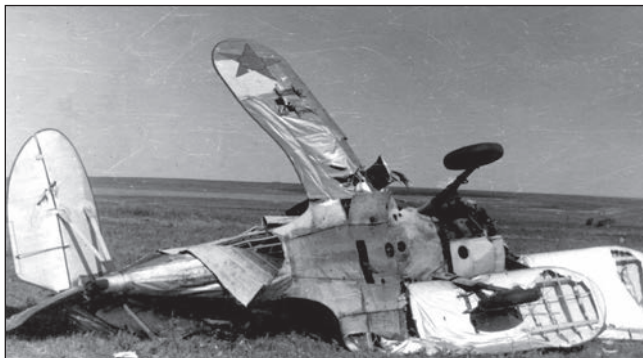
Left: I-15bis from the 55th Fighter Aviation Regiment (IAP, Istrebitelnyy Aviatsionnyy Polk ) destroyed by Luftwaffe at Beltsi airfield. It is clearly visible that the undersides of the fuselage and wings are painted with АПАЛ silver (aluminum) aircraft lacquer.
