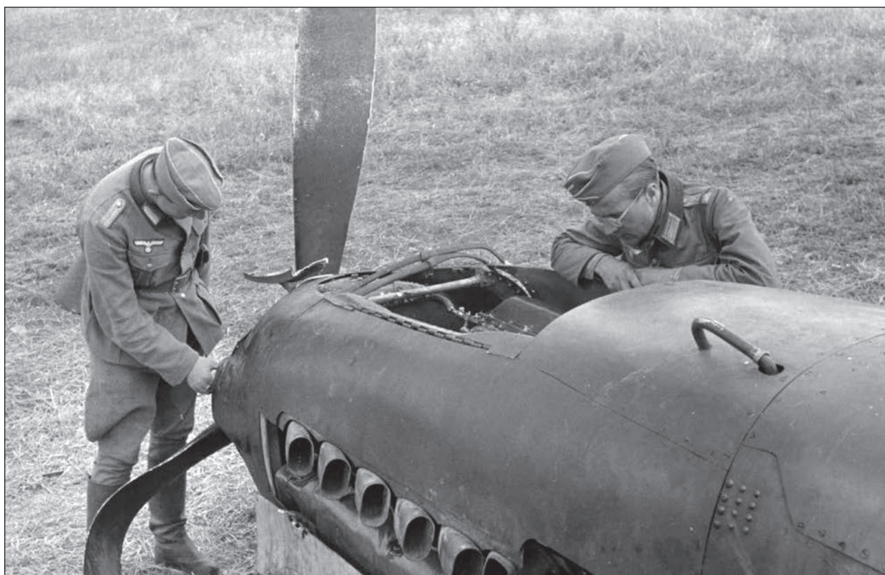
Il-2 of an unknown unit, captured by the enemy at the place of forced landing, August–September 1941. The airplane was painted in improvised black-and-green camouflage, with alternating colours and insignia in six positions – four of increased size and the stars on the tail fin of the earlier (smaller) size.
