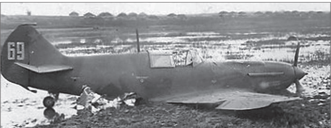
LaGG-3, tactical number 69, manufactured by Factory No.31. The airplane was painted in black-and-green standard camouflage – the AMT-4 and AMT-6 paints were used for the upper surfaces, and the AMT-7 light blue for the undersides. This airplane of an unknown unit was captured by the enemy at the site of forced landing.
