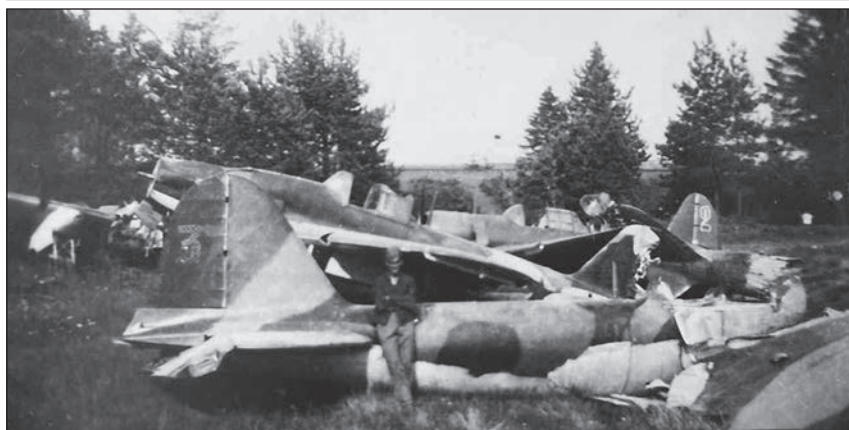
Il-2, tactical number 3, presumably from the 61st ShAP photographed by German soldiers at Shatalovo airfield. The airplane was painted in black-and-green camouflage according to the scheme attached to SNK Directive No.1711, the insignia applied in four positions (wing undersides and vertical tail).
