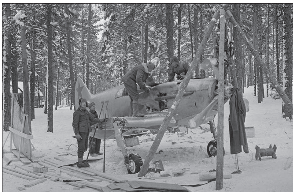
LaGG-3, tactical number 33, presumably built by the Factory No.23. The aircraft was discovered on 20 February 1942 in the vicinity of Vidlitsa (35km to the north of Olonets) and captured by Finnish troops. Later it was restored and used in the Finnish Air Force with LG-2 registration number.
