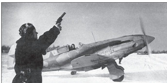
Left and below: MiG-3 of the 6th IAK of the Air Defense Forces, winter 1941–42. The airplane upper surfaces were painted in white throughout, the enlarged insignia were applied in six positions.
