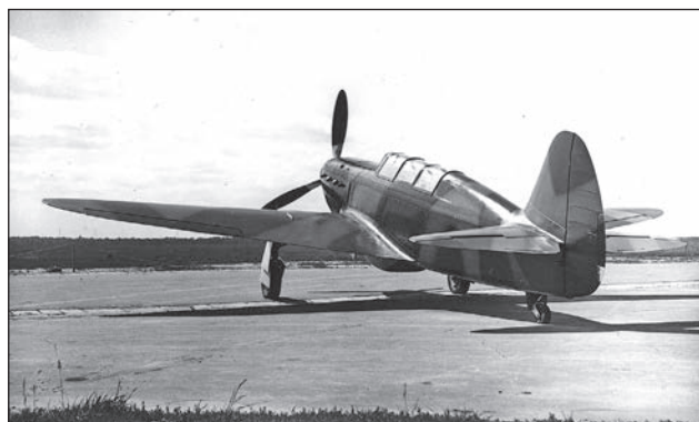
UTI-26-I during factory tests on 23–25 July 1940. Yak-7 (UTI-26) became the first serial aircraft of the VVS RKKA painted in two-colour black-and-green camouflage.
