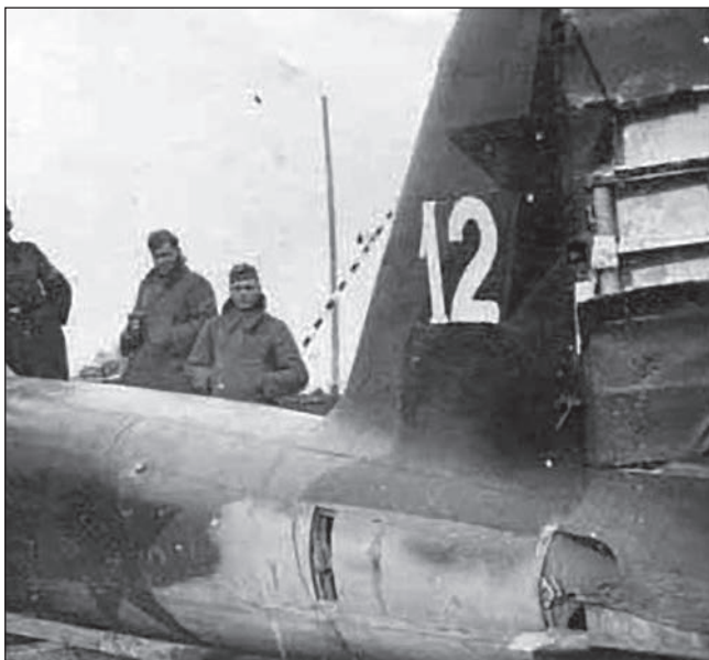
Il-2 tactical number 12, of an unknown unit, captured by the enemy at the place of forced landing, July–August 1941. The airplane was painted in the improvised black-and-green camouflage, with alternating colours and enlarged insignia in six positions.
