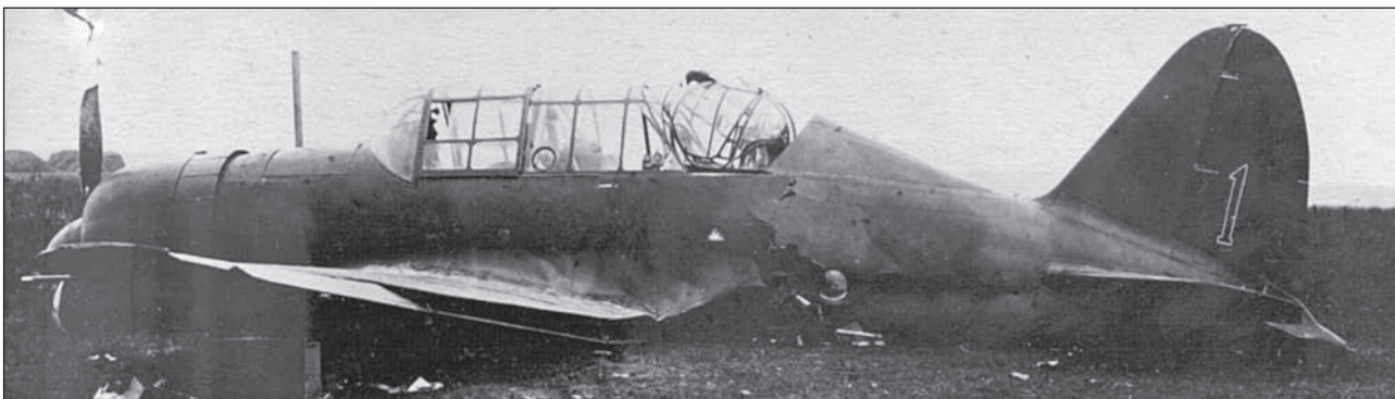
Su-2, tactical number 1, of the 43rd BAP, after forced landing, August 1941. The aircraft was painted in black-and-green camouflage, with insignia applied in six positions according to the improvised scheme of Factory No.135.
