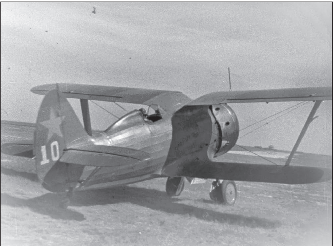
I-153 of the 160th IAP after overhaul at Factory No.1. The airplane was painted green overall on upper surfaces, insignia placed in four positions (wing undersides and vertical tail), according to the scheme attached to the SNK Directive No.1711.
