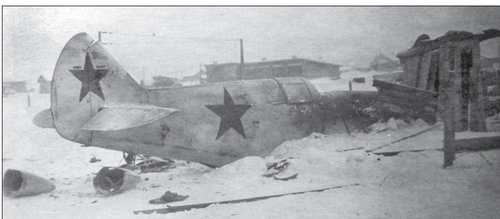
Crash of the LaGG-3 s/n 312119-21 at the airfield of Factory No.21 due to the engine failure during the acceptance test flight on 25 January 1942.
