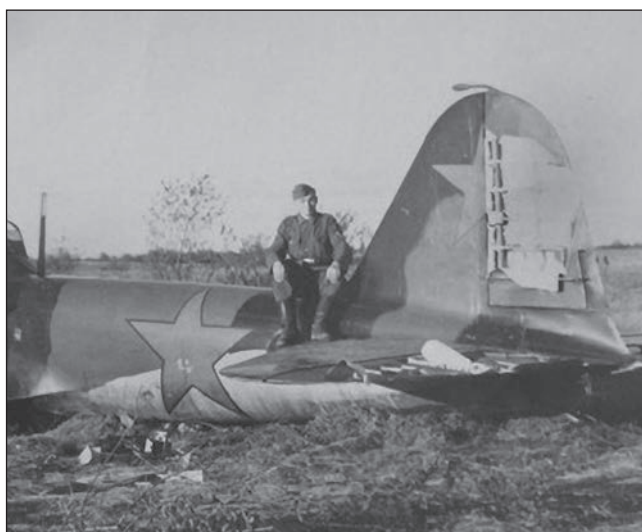
Il-2 of an unknown unit, captured by the enemy at the place of forced landing, August–September 1941. The airplane was painted in improvised black-and-green camouflage, with enlarged insignia applied in six positions.
