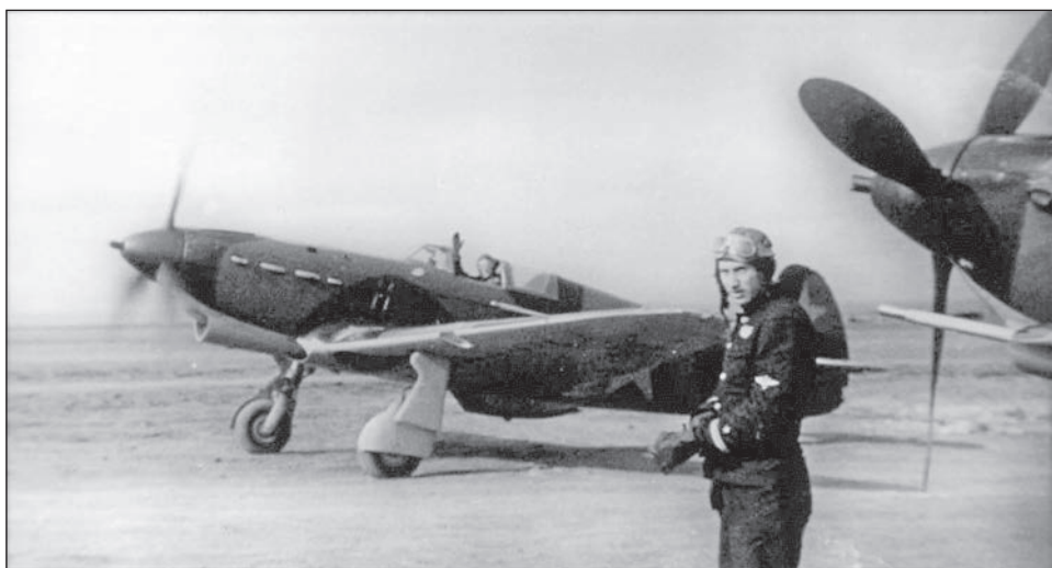
Yak-1 from the 1st Squadron of the 8th IAP of the Black Sea Fleet Air Force, spring 1942. The airplane was painted in black-and-green camouflage, according to the scheme attached to the SNK Directive No.1711, with enlarged insignia applied in six positions.
