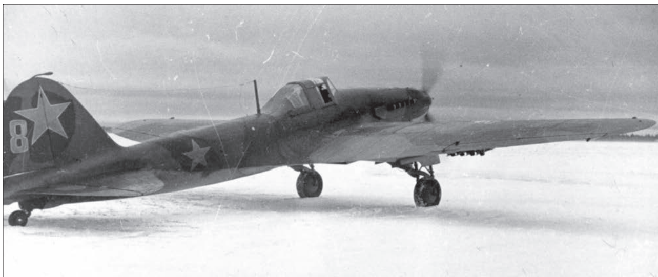
Il-2, tactical number 8, of the 174th ShAP, autumn 1941. The airplane was painted in improvised black-and-green camouflage, the insignia with white edging applied in six positions, and a star of reduced size on the fuselage.
