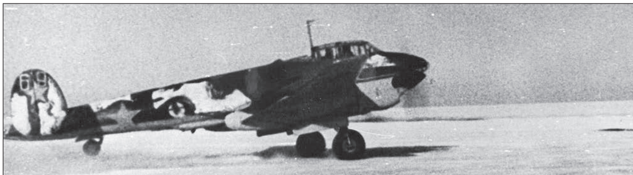
Pe-2 bomber, tactical number 69, from the 5th SBAP of the Southern Front Air Force. The airplane was painted in the improvised winter camouflage of irregularly shaped white spots over the basic black-and-green camouflage, winter 1941–42.
