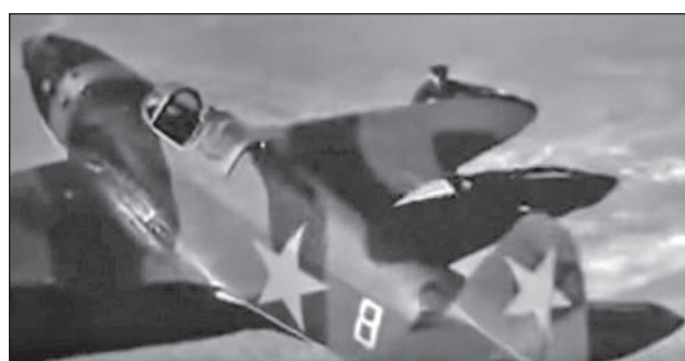
Yak-1, tactical number 8, from the 8th IAP of the Black Sea Fleet Air Force, spring 1942. The airplane was painted in black-and-green camouflage, according to the scheme attached to the SNK Directive No.1711, in alternating colours with enlarged insignia applied in six positions.
