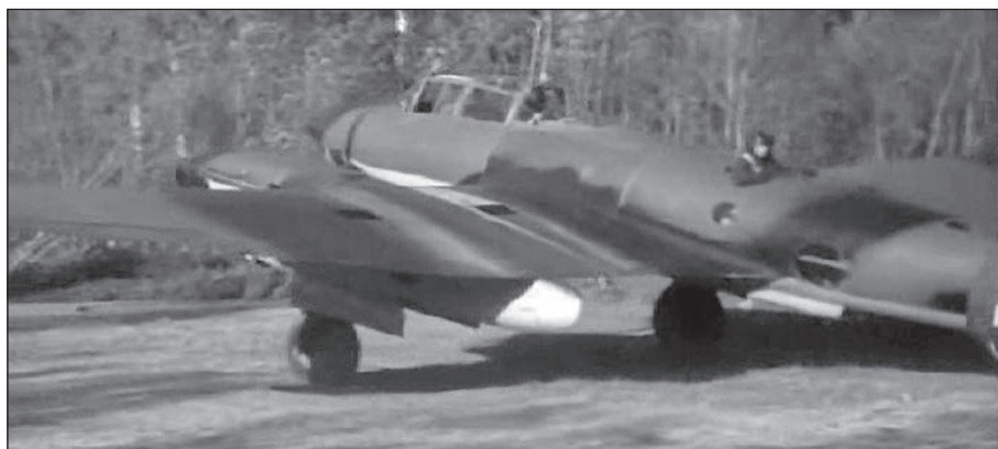
Pe-2, tactical number '5 white' (airplane of the 29th series of Factory No.22), from the 260th BAP of the 6th Composite Aviation Division (SAD, Smeshannaya Aviatsionnaya Diviziya ), August 1941. The airplane was painted in black-and-green camouflage, with insignia applied in four positions (on the wing undersides and on the vertical tail) according to the scheme attached to SNK Directive No.1711; the stars on the vertical fins are of enlarged size.
