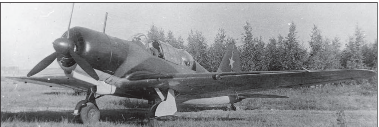
Su-2 in artillery spotter version during tests in August 1941. The airplane was painted in black-and-green camouflage, insignia were applied in four positions (wing undersides and vertical tail), according to the scheme attached to the SNK Directive No.1711.
