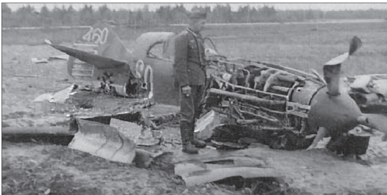
LaGG-3 built by Factory No.21, tactical number 460. The airplane was painted in black-and-green camouflage, according to the scheme attached to the SNK Directive No.1711. The AMT-4 and AMT-6 paints were used for the upper surfaces, and the AMT-7 light blue for the undersides. The insignia of the increased size were applied in six positions. The airplane was captured by the enemy at the place of forced landing. The fighter presumably belonged to the 46th IAP, 8th IAD, August–September 1941.
