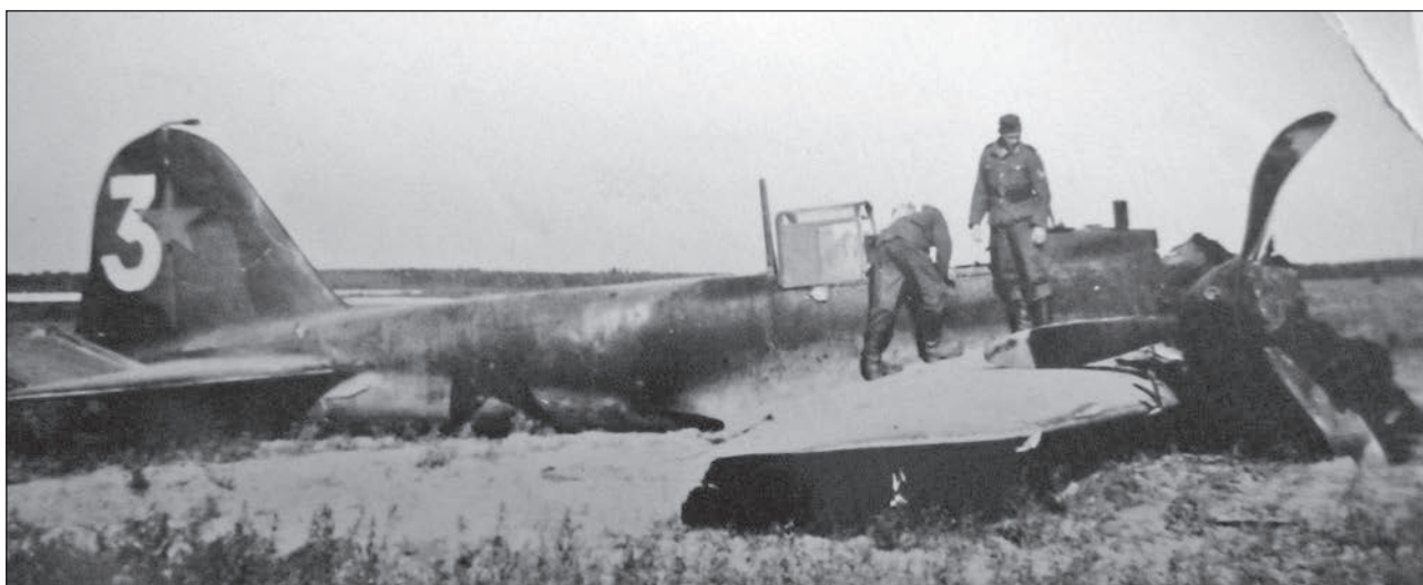
Il-2, tactical number 3, of an unknown unit, captured by the enemy at the place of forced landing, August–September 1941. The airplane was painted in improvised black-and-green camouflage, with insignia in six positions – four of increased size and the stars on the tail fin of the earlier (smaller) size.
