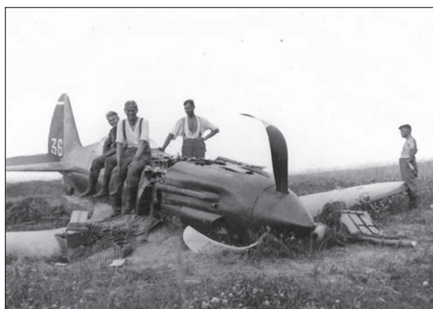
MiG-3 fighters manufactured by Factory No.1 in June 1941. Insignia on fuselages and wing upper surfaces were painted over, the stars on the wing undersides were enlarged, stars on the vertical tail were applied according to the scheme attached to the SNK Directive No.1711.
