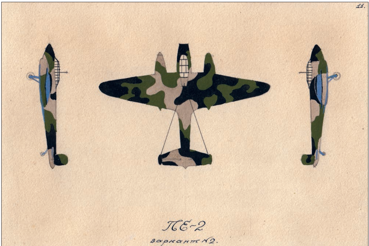
Camouflage scheme of Pe-2 bomber. Variant No.2.
