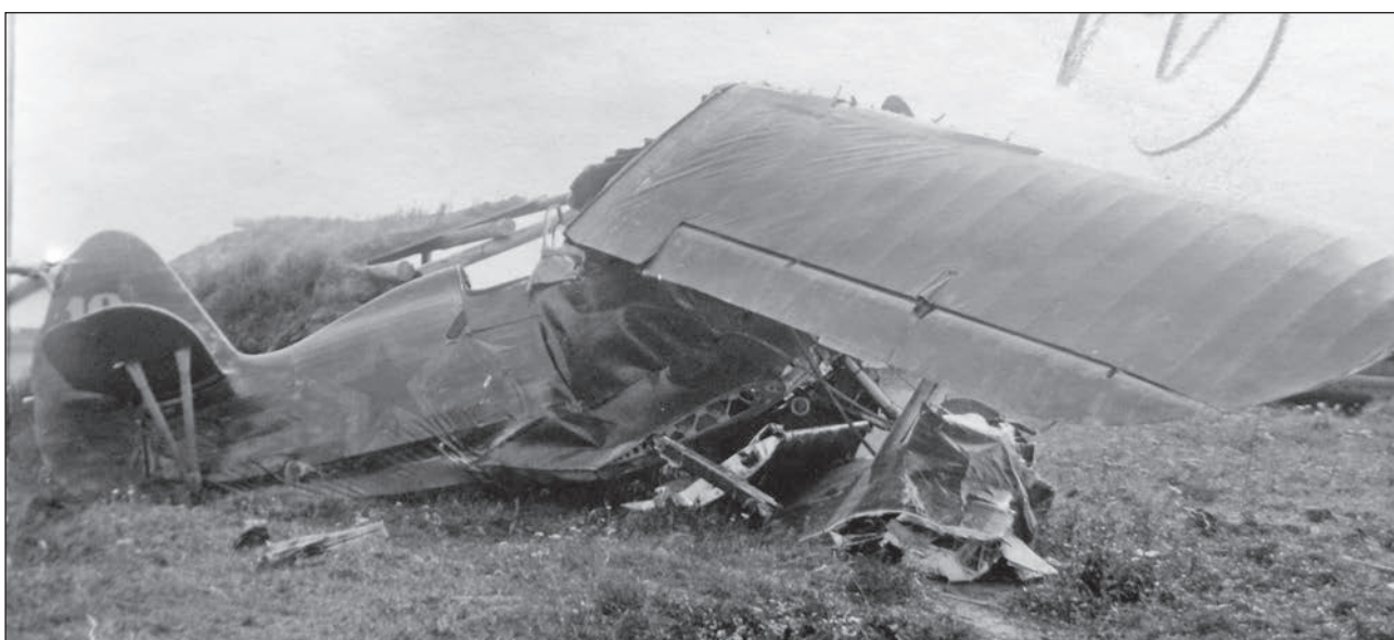
I-153 s/n 6853, tactical number 12, from the 4th Squadron of the 152nd IAP. On 10 August 1941, the fighter flown by the Wing Commander, Lieutenant I.N. Galoshin crashed at Kegostrov airfield. The airplane had been repainted – the upper surfaces in green, the undersides in blue, the insignia on the wing upper surfaces were painted over, but on the vertical tail they were not applied at all. (24).
