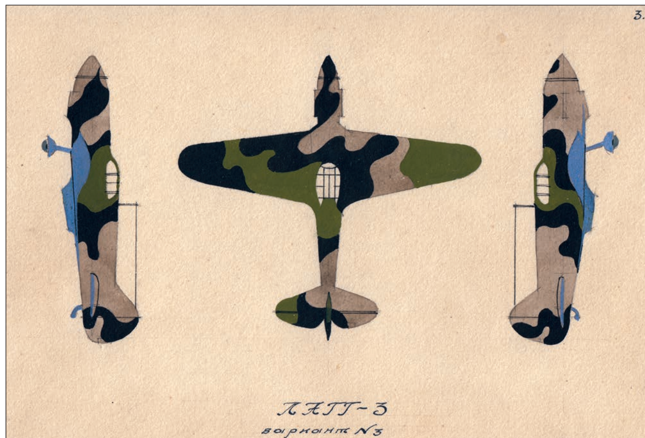
Camouflage scheme of LaGG-3 fighter. Variant No.3.
