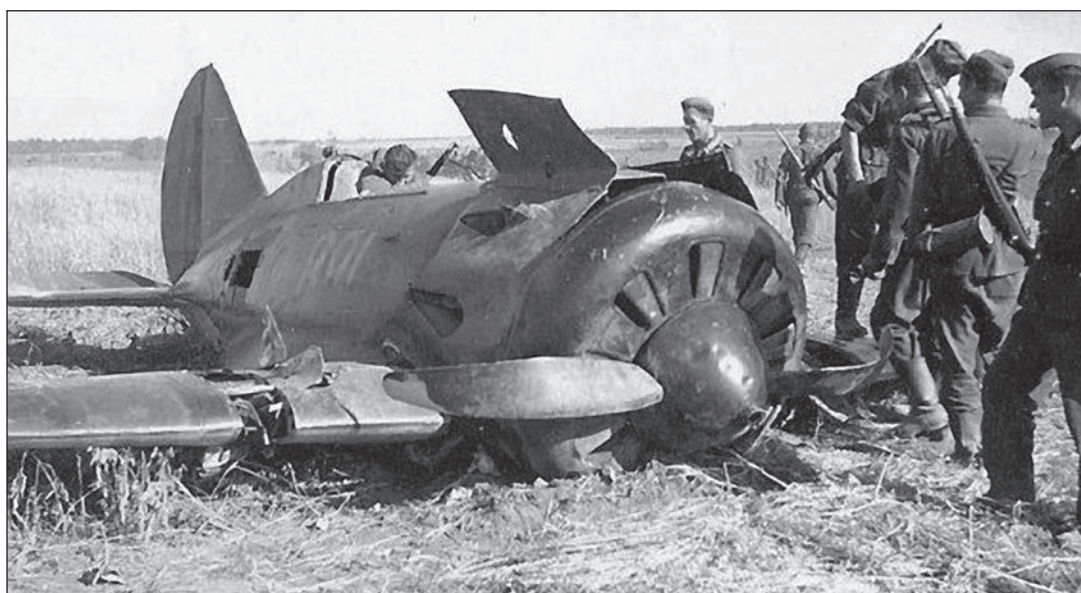
I-16 type 5 s/n 521894, tactical number 894, from the 154th IAP of the 39th Fighter Aviation Division (IAD, Istrebitelnaya Aviatsionnaya Diviziya ) after a forced landing. The fighter was painted in improvised black-and-green camouflage with insignia applied in six positions according to the pre-war standard.
