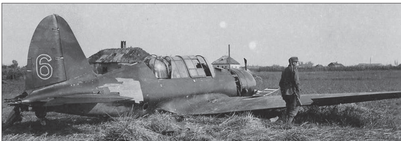
Su-2, tactical number 6, of an unknown unit, captured by the enemy at a forced landing site, August–September 1941. The airplane was painted in black-and-green camouflage, with insignia applied in six positions according to the improvised scheme of Factory No.135.
