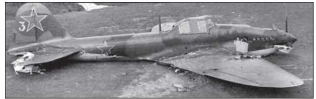
Il-2, tactical number 3, manufactured at the end of summer 1941, painted in improvised black-and-green camouflage. The vertical tail still had a horizontal black stripe of irregular shape, insignia with white edging applied in six positions, and a star of reduced size on the fuselage.
