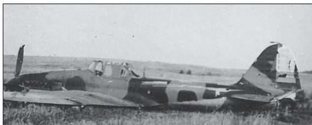
Il-2s presumably from the 74th ShAP, painted in black-and-green camouflage according to the scheme attached to the SNK Directive No.1711, with insignia applied in four positions (wing undersides and vertical tail), photographed by German troops at the sites of forced landings.
