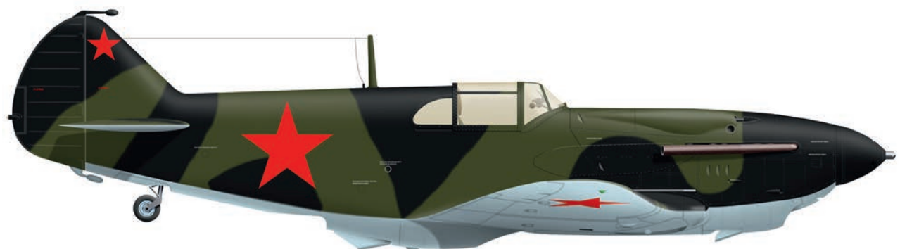
Scheme of camouflage painting of the LaGG-3 airplanes was implemented at Factory No.31 in late June 1941. It was compiled according to the scheme attached to the SNK Directive No.1711 – the AMT-4 and AMT-6 paints were used for the upper surfaces, and the AMT-7 light blue for the undersides; propeller blades were painted in AM-26 black. Insignia applied in six positions – on the wing undersides, the fuselage and the vertical tail with red nitro lacquer II.
