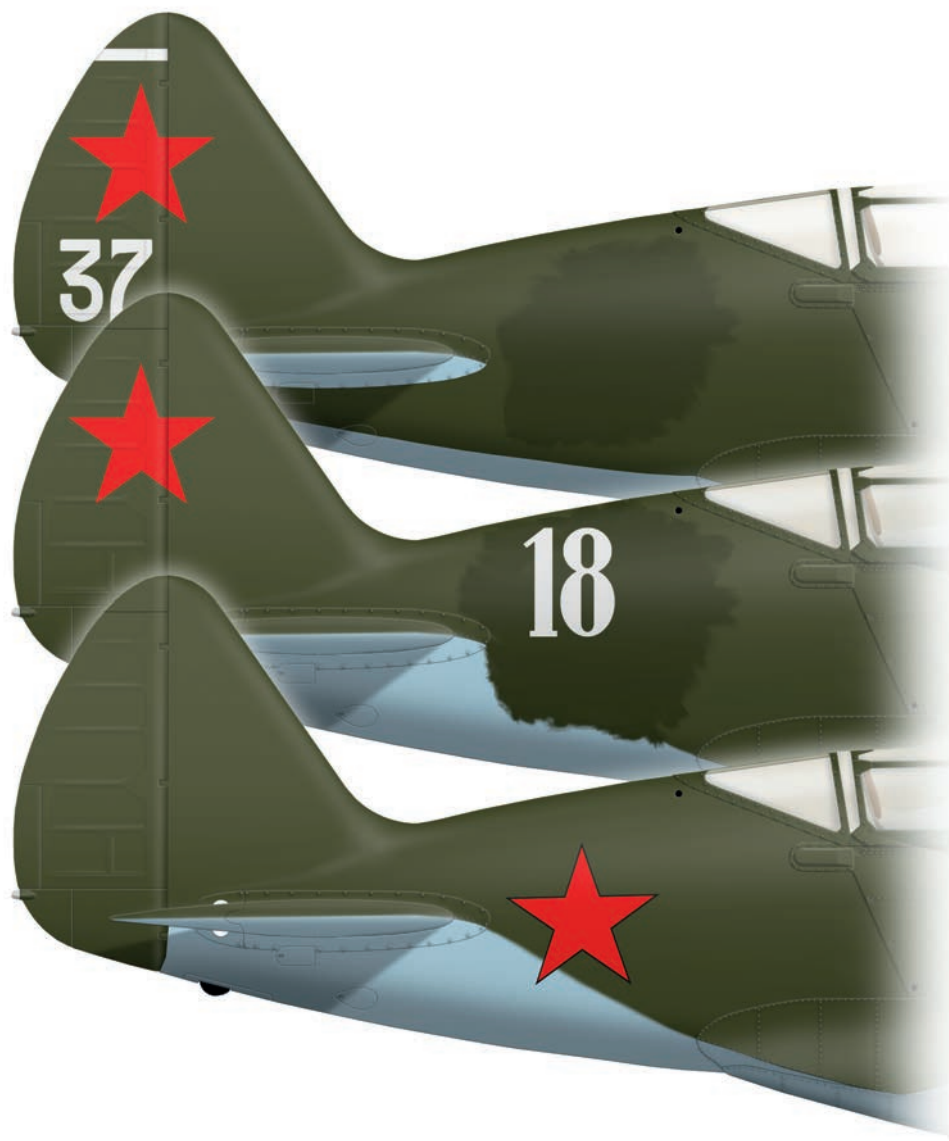
Tail parts (two upper views) of MiG-3s manufactured by Factory No.1 in June – early July 1941. Insignia on fuselages and wing upper surfaces were painted over, the stars on the wing undersides were enlarged, the stars on the vertical tail were applied according to the scheme attached to the SNK Directive No.1711. For comparison, the lower view shows the tail part in a standard pre-war colour scheme and insignia on the fuselage.
