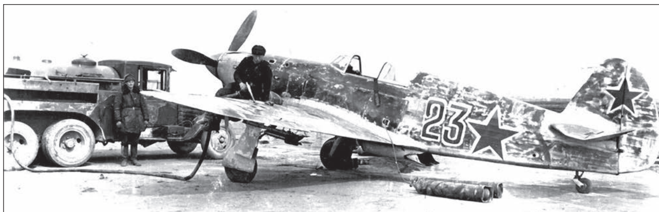
Yak-1 s/n 0506 from the 123rd IAP of the 7th IAK of the Air Defense Forces, flown by Captain G.N. Zhidov, 23 April 1942. The wear of winter camouflage is clearly seen, the paint on the nose part is almost completely peeled off.
