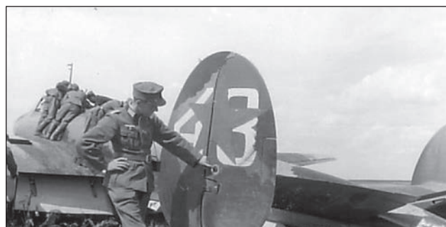
Pe-2 of the early series built by Factory No.39, tactical number 48, of the 5th SBAP, which crash-landed near Babanka (Uman region) in August 1941. The airplane was painted in black-and-green camouflage with insignia applied in four positions according to the scheme attached to the SNK Directive No.1711.
