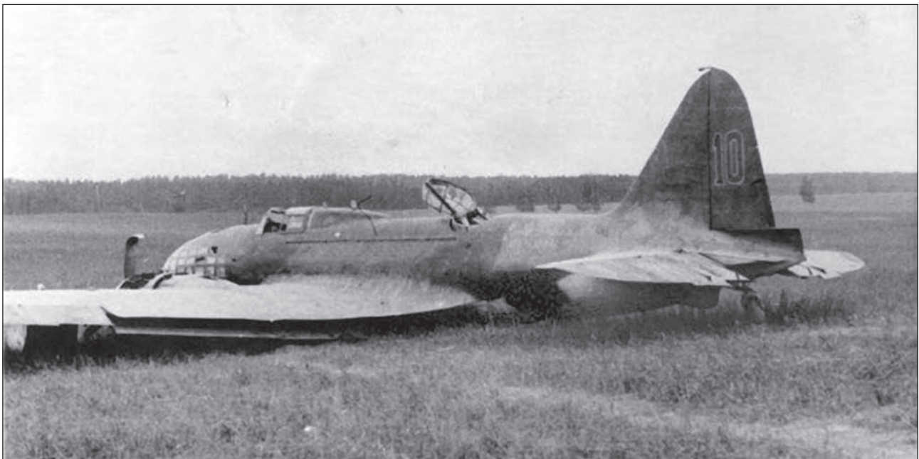
DB-3f, tactical number 10, of an unknown unit was shot down and landed at the enemy's territory. The airplane was painted in improvised camouflage of small black spots, insignia on the fuselage and wing upper surfaces were painted over, stars on the vertical tail were painted according to the scheme attached to the SNK Directive No.1711.
