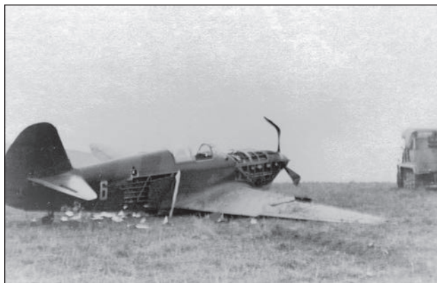
Yak-1 s/n 0636, tactical number 6, captured by the enemy at the place of forced landing, Crimea 1941. Aircraft painted in black-and-green camouflage, according to the scheme attached to the SNK Directive No.1711, insignia of enlarged size are applied in six positions.
