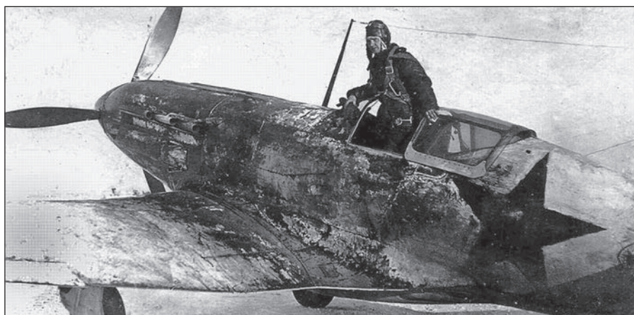
Yak-1 s/n 0506 from the 123rd IAP of the 7th IAK of the Air Defense Forces, flown by Captain G.N. Zhidov, 23 April 1942. The wear of winter camouflage is clearly seen, the paint on the nose part is almost completely peeled off.
