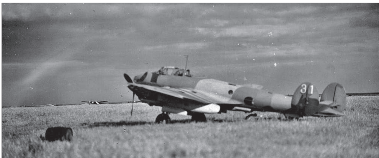
Pe-2 of the 5th SBAP near Odessa, summer 1941. The airplane was manufactured after 20 June 1941, painted in experimental three-colour camouflage with insignia applied in four positions – on the wing undersides and on the vertical tail.
