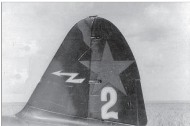
Su-2, tactical number 2, presumably from the 226th Short-Range BAP, captured by the enemy at the place of forced landing, summer 1941. The airplane was painted in black-and-green camouflage and carried insignia in four positions according to the scheme attached to the SNK Directive No.1711. Note that the star on the rudder is already of enlarged size.
