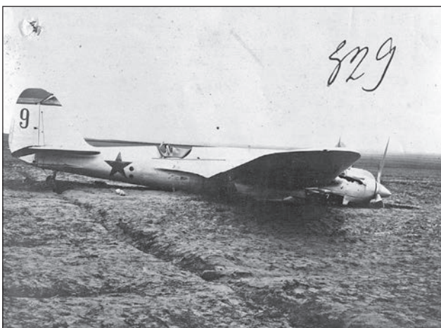
SB bomber s/n 8/217 of the 24th SBAP remained in standard colour of AE-9 light grey enamel.
