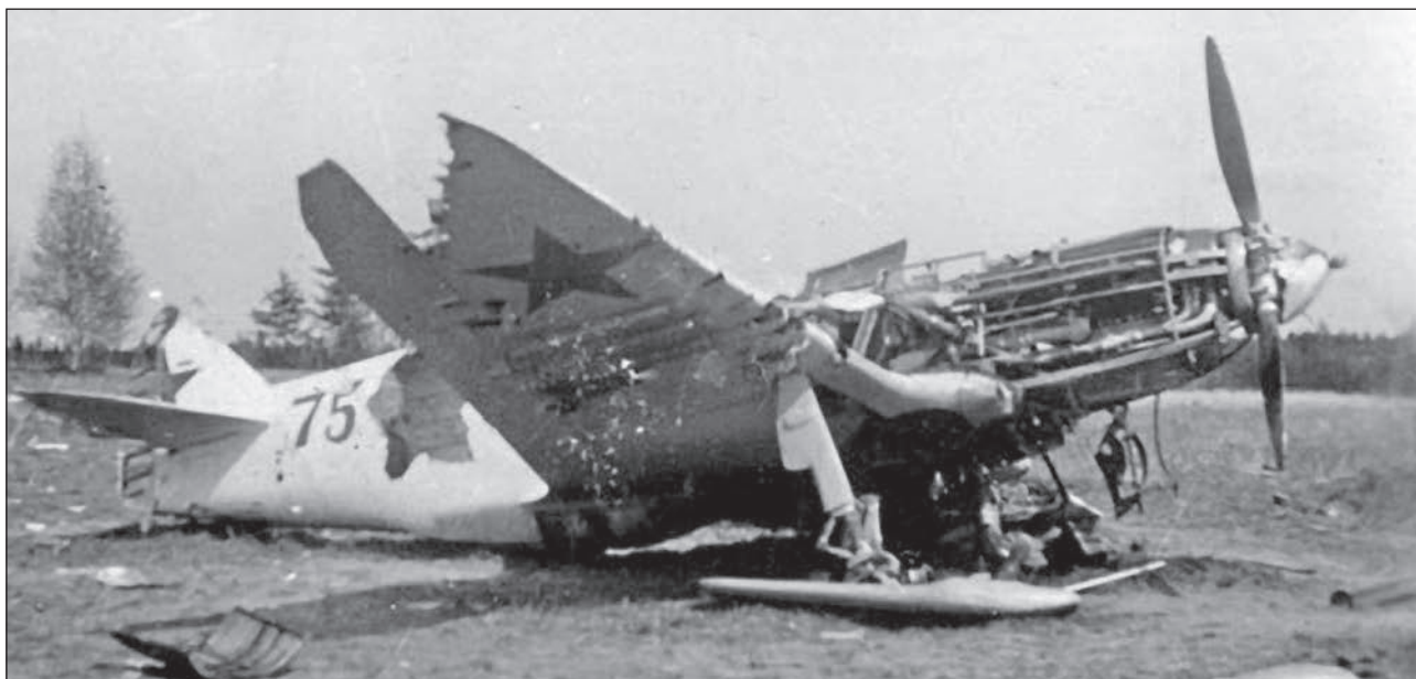
LaGG-3, tactical number 75, of an unknown unit, captured by the enemy at the place of forced landing, March 1942. Note that the aircraft is still equipped with ski landing gear.
