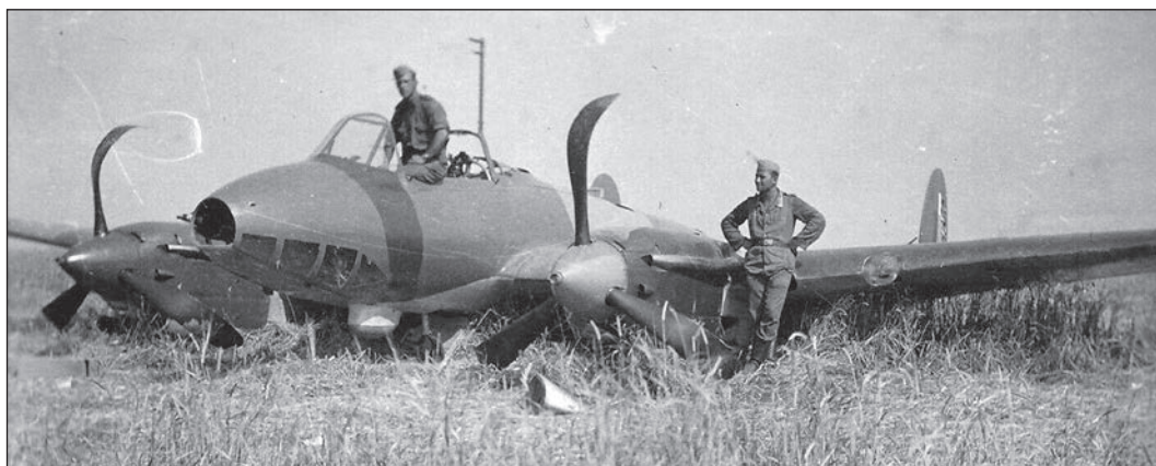
Pe-2s of an unknown unit, pictured by the enemy at forced landing locations, summer 1941. The aircraft were painted in experimental three-colour camouflage with insignia applied in four positions – on the wing undersides and on the vertical tail.
