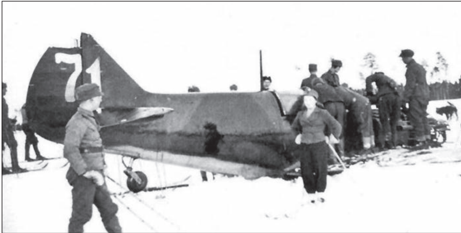
LaGG-3, tactical number 71, of the 524th IAP, captured by Finnish soldiers at the place of forced landing in winter 1941–1942. The airplane was painted in black-and-green camouflage, with alternating colour spots. The insignia applied in six positions with an enlarged star on the vertical tail.
