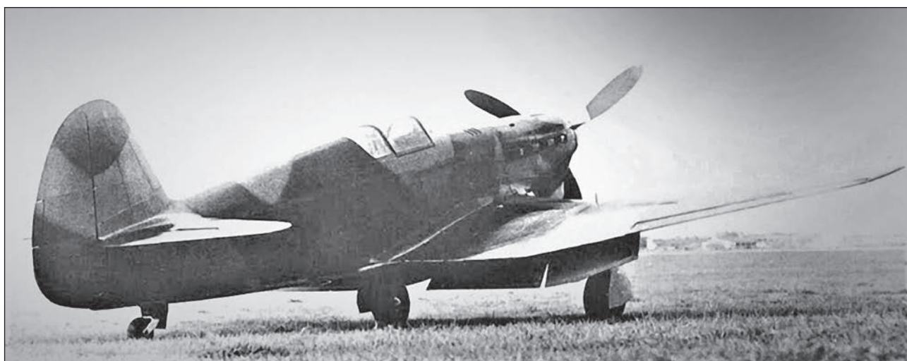
A prototype of I-30 fighter (the first and second prototypes) in characteristic experimental camouflage during factory testing, 1940–1941.
