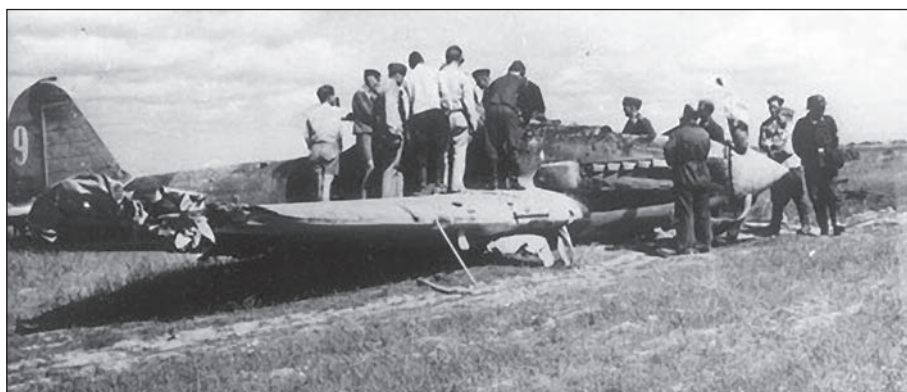
Il-2, tactical number 9, of an unknown unit, captured by the enemy at the place of forced landing, July–August 1941. The airplane was painted in improvised black-and-green camouflage, with alternating colours and insignia in six positions – four of increased size and the stars on the tail fin of the earlier (smaller) size.
