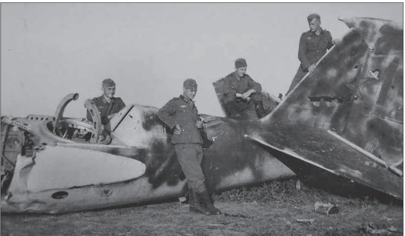
SB bombers, tactical numbers 1 and 6, of an unknown unit, were shot down in air combat or by enemy anti-aircraft fire. The airplanes were painted in the so-called 'Khalkhin-Gol' camouflage, the insignia on the fuselages and on the wing upper surfaces were painted over, the stars on the vertical tail were applied according to the scheme attached to the SNK Directive No.1711.
